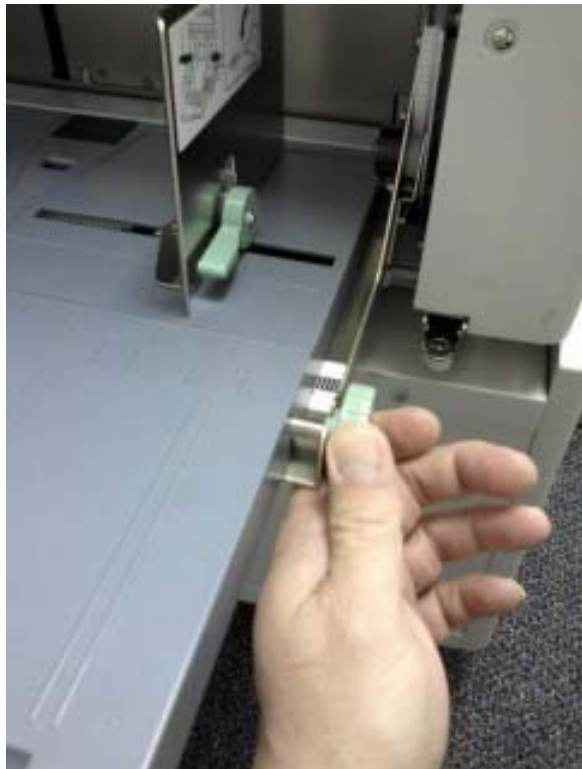
The user can also adjust the input-paper tray's position to the right or left to facilitate more accurate feeding of paper.
