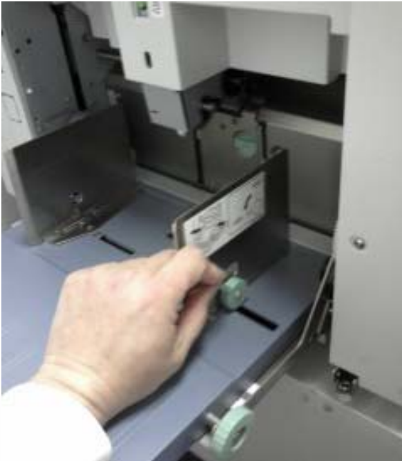
The user slides this guide into position in order for the paper-input tray to accommodate different paper sizes.
