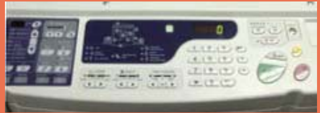
The EZ390 incorporates a control panel consisting of hard keys and an LED panel (no touch screen).
