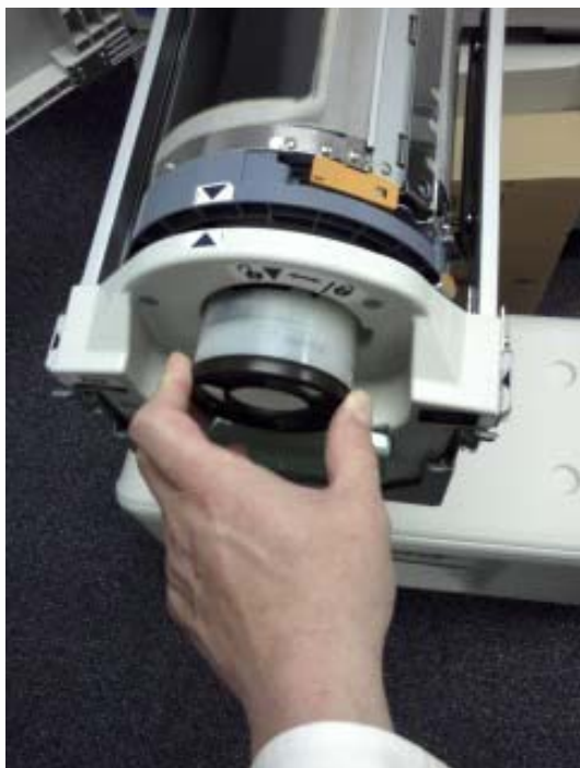
Above and below: Ink is contained in a cylinder that is easy to remove and replace.
