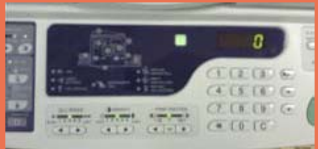
The center of the control panel contains the LED panel, numerical keypad for entering number of copies, and a graphic of the device that lights up to indicate various device components.
