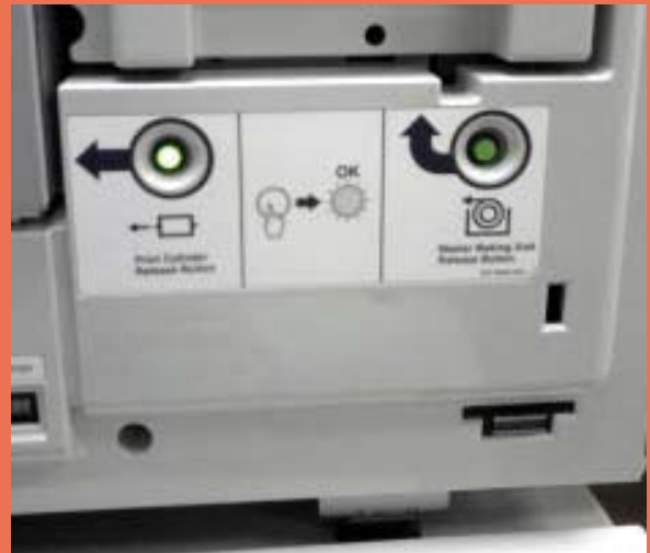
In order to remove either the master roll or imaging drum, the user presses a button to release either of the units, pressing the button on the right to release the master unit, and pressing the button on the left to release the imaging unit. Once the light within the button is green, the units can safely be removed.
