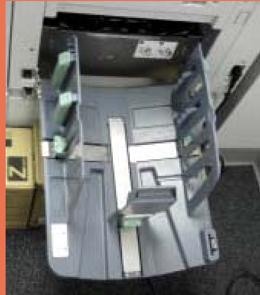
Above and below: The EZ390's standard paper-output tray that can hold up to 1,000 printed pages.
