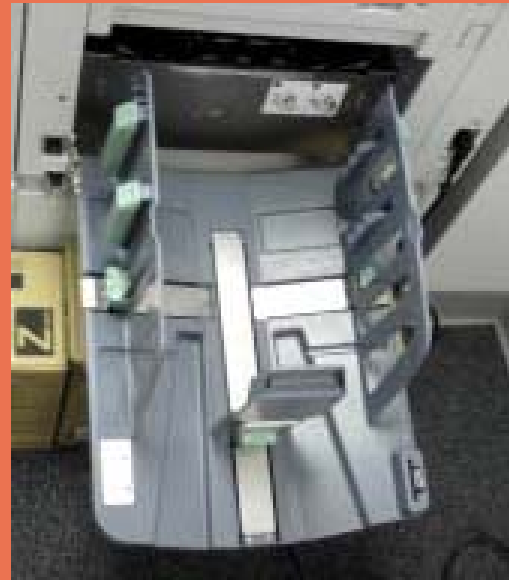
Above and below: The EZ220's standard paper-output tray that can hold up to 1,000 printed pages.
