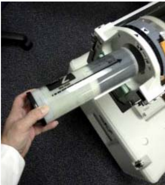
Above and below: Ink is contained in a cylinder that is easy to remove and replace.
