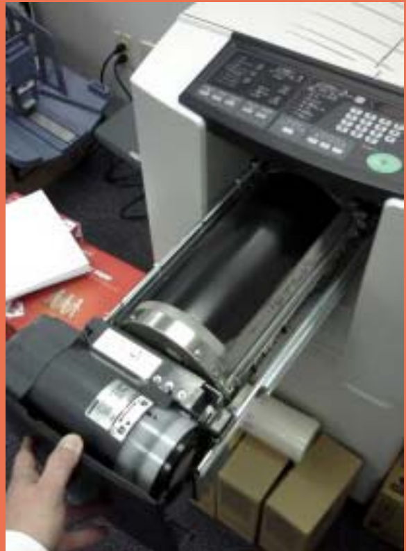
The ink cylinder is located in the bottom left of the photo above.
