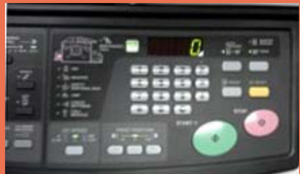
The center of the control panel contains the LED panel, numerical keypad for entering number of copies, and keys for master-making, printing, printing a proof page, resetting selections, and adjusting the image's position.
