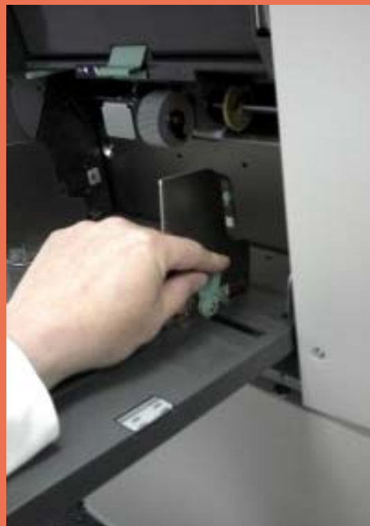
The user slides this guide into position in order for the paper-input tray to accommodate different paper sizes.
