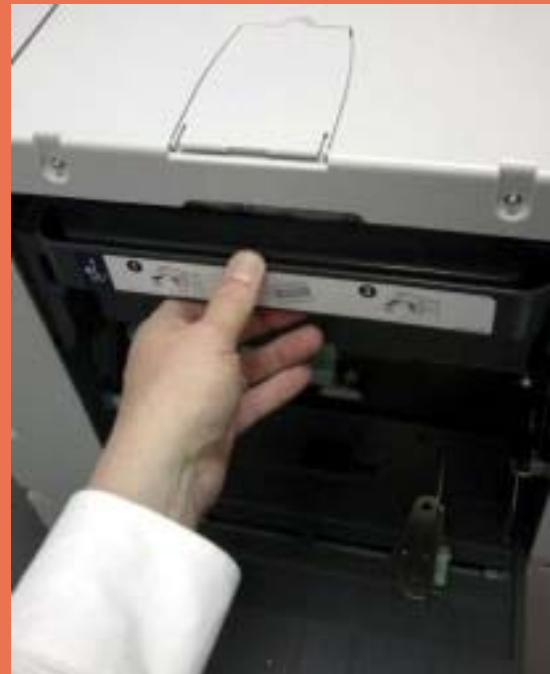
The master disposal box, which contains used, inked masters, is located on the left side of the unit.
