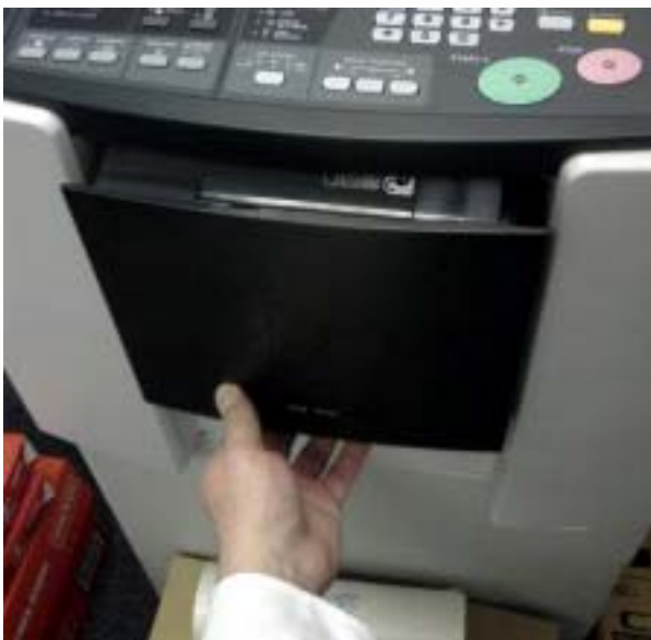
In order to access the imaging drum and ink container, the user first opens the front drawer as shown above, pulling out the imaging drum and ink cylinder (next photo).
