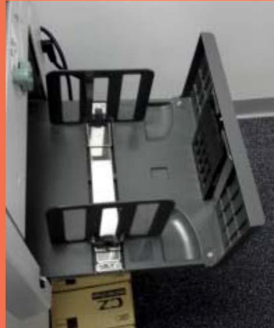
The CZ180's standard paper-output tray, located on the right side of the unit, can hold up to 800 printed pages.
