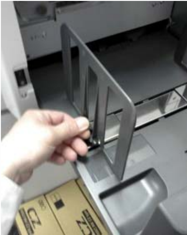
Adjusting the CZ180's paper-output tray to accommodate different paper sizes. Users simply slide the guides into position as shown above.
