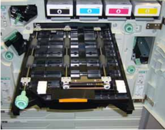
The duplex and paper transport units pull out like a drawer for easy access to misfeeds.
