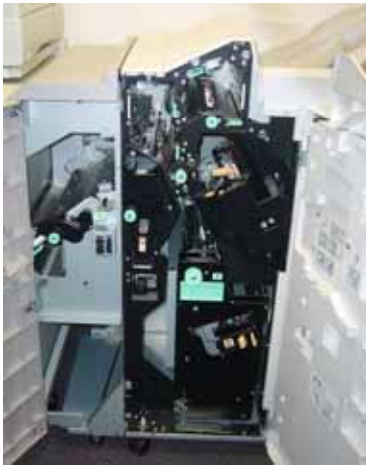
Users have access to the misfeed areas on the Multifunctional Finisher by simply opening the front doors of the finisher and following the instructions on the control panel to locate the specific section where a jam has occurred.
