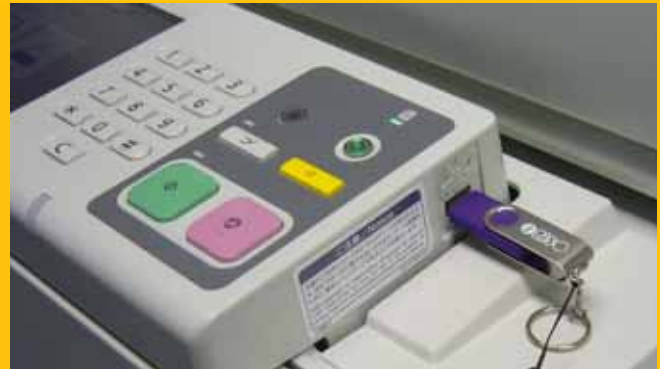
The ComColor 7010 comes standard with a USB port for storing scanned data. Users can save scan files as either a PDF, TIFF, or JPEG.
