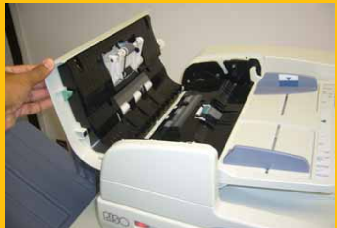
Above and below: The RISO ComColor 7010's platen (above) and document feeder (below), with the document feeder's cover opened in order to expose the feeder's misfeed-access area.
